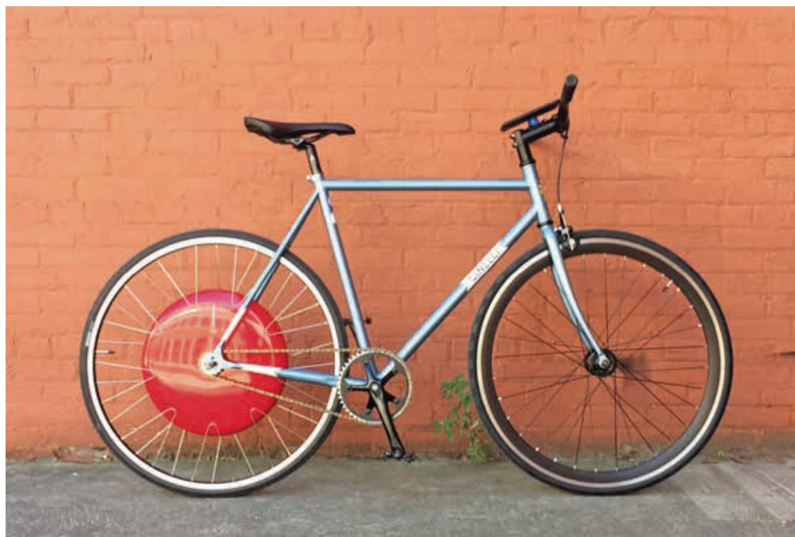
A basic e-bike setup is this red hub mounted onto a traditional bicycle frame. The Copenhagen Wheel, produced by Superpedestrian, is controlled by an app on the rider's smart phone, and it makes pedaling the bike up hills or across town a breeze.
